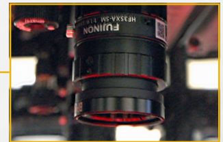
CMOS camera & machine vision lens; Customized magnification configurations
